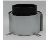
The MT5 collar is placed around the synthetic pipe. It must be placed applied. Easy placement by removing the slides, opening the sleeve, placing on the pipe and replacing the slides. The free air passage is 100% and the fire resistance can go up to 120min.
