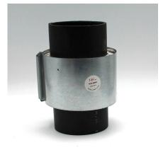
The MT4 collar is placed around the synthetic pipe. It must be recessed. Easy placement by removing the slides, opening the sleeve, placing on the pipe and replacing the slides. The free air passage is 100% and the fire resistance can go up to 120min.
