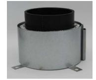
The MT5 collar is placed around the synthetic pipe. It must be placed applied. Easy placement by removing the slides, opening the sleeve, placing on the pipe and replacing the slides. The free air passage is 100% and the fire resistance can go up to 120min.
